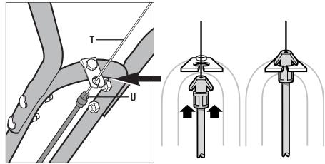
Fig. 2-4: Installing forward clutch cable bracket and cable.
